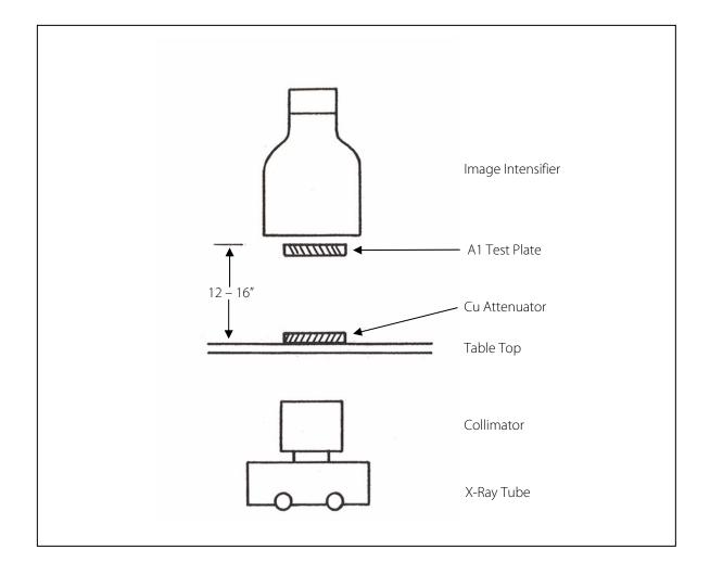
Figure 1-1. Fluoro-Test Threshold Contrast Resolution Imaging Geometry.
