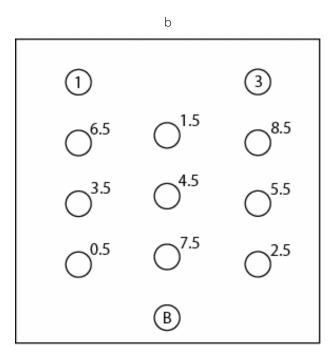
*Figure 1-2B.* Test object numbered to indicate calibrated contrast at 80 kVp for the Half-Integer *Phantom.*
